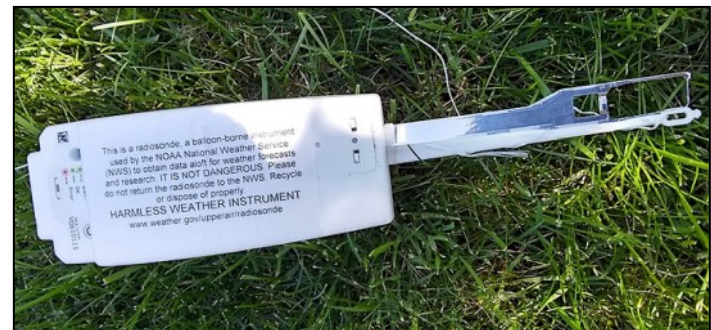
Info & instructions printed on Radiosonde RS41.
